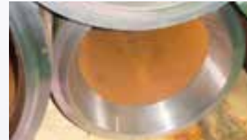
Pipe material nine-crome, 750 mm OD
